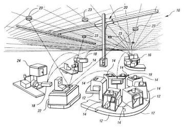
Fig. 4. An example of structure of Reconfigurable Manufacturing System [13]
