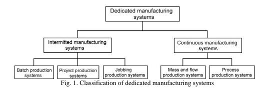
When analyze the flexibility level of dedicated manufacturing systems, it is worth to notice that continuous manufacturing systems are typically rigid where the level of flexibility is around "zero". The intermittent systems, where the need of flexibility has been already noticed, are designed as a "customer focused", taking into account the problem of variation and changeability of customers' orders.
