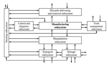
Fig. 3. A functional structure of an FMS [11]
