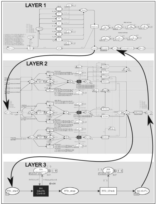
Considering the feature of hierarchical Petri net, the whole model was divided into three layers, shown in figure 3 along with flow directions of production orders.
