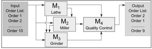
Fig. 1. Simplified schematic diagram of a production system
