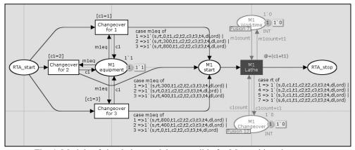
Fig. 4. Module of simulation model responsible for M1 machine changeover
