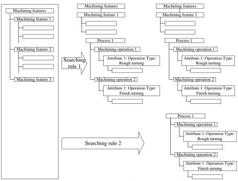
Fig. 3. Effect of adding alternative machining operations using searching rules
