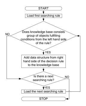
Fig. 2. The working principle of searching rule
