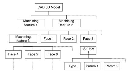
Fig. 1. Hierarchical structure representing machining features and their parameters
