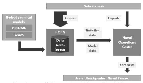
Fig. 1. Oceanographic Support Information System of the Polish Navy
