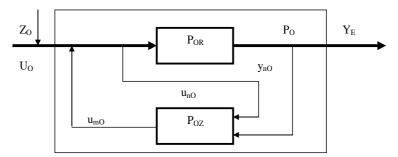
Fig. 4. The idea of machinery exploitation management in an enterprise:  $P_{OR}$  – exploitation working subsystem,  $P_{OZ}$  – exploitation management subsystem,  $U_O$  – input,  $Y_O$  – outputs,  $Z_O$  – disruptions,  $u_{no}$ ,  $y_{no}$ ,  $u_{mo}$  – signals: input, output and steering respectively
