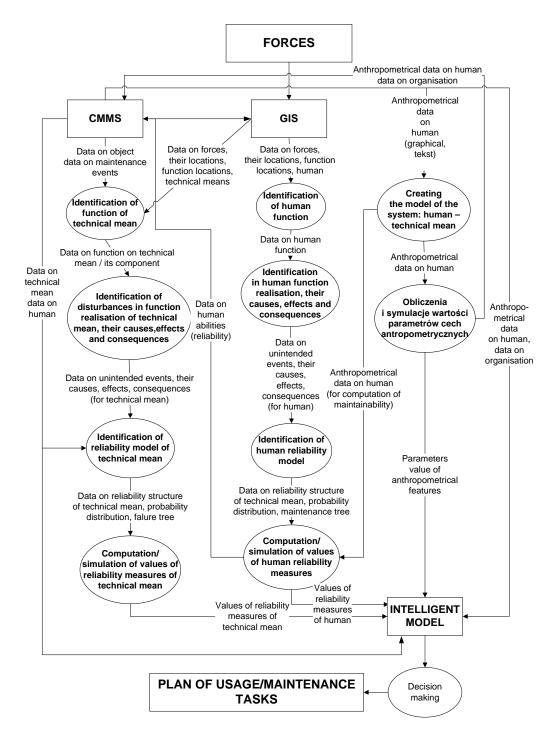
Fig. 3. DFD (ang. Data Flow Diagram) model of the feature of the system: human – technical mean – environment
