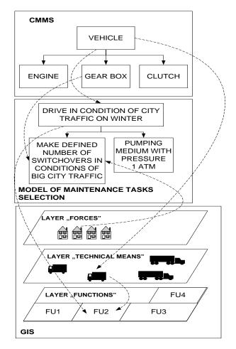
Fig. 9. Connection between functions with object/their components (CMMS) and layers of maps (GIS)
