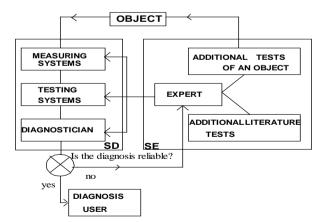
Fig. 5. IT connections in a diagnostic export system
