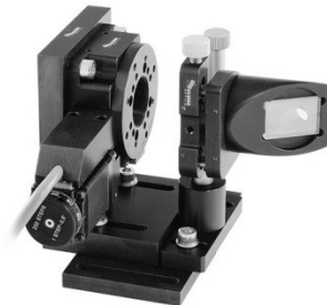
Fig. 12. Motorized variable attenuator for linearly polarized laser beam [8]
