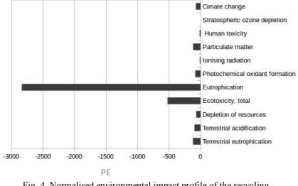
Fig. 4. Normalised environmental impact profile of the recycling process of dry waste in Kielce Source: Own research
