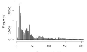
Test case durations [s] Fig. 2. Histogram of execution times of test cases
