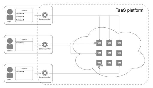
Fig. 1. Structure of considered TaaS system, showing clients, test suites, local dispatchers, cloud resources and submitting of test cases
