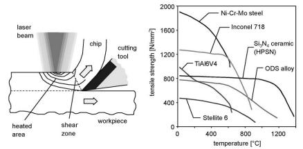
Fig. 5. Principle of laser assisted machining (left) and effect of temperature on the ultimate tensile strength for various hard-to- machine materials (right) [9].
