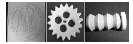
Fig. 2. The complex-shaped sintered Al2O3 ceramic parts prepared by laser-machining [5]
