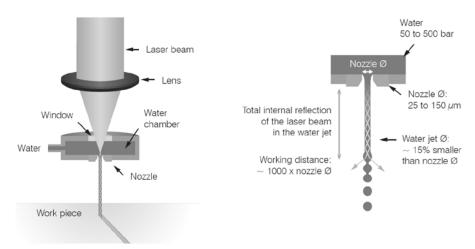
Fig. 8. The scheme of water jet guided laser technology [13]
