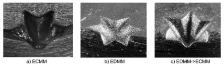
Fig. 10. Photographs of cavities machined during electrochemical sinking (a), electrodischarge sinking (b) and sinking when using the EC/EDMM sequence (c) [14].
