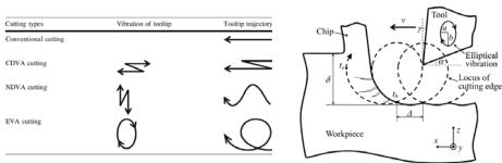
Fig. 6. Cutting types (a) and schematic illustration of vibration assisted cutting (b)
