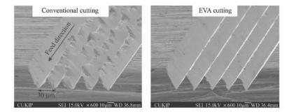
Fig. 7 Image of micro v-grooves machined by conventional cutting (left) and vibration assisted cutting (right) [12]
