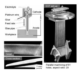
Fig. 4. Electrochemical Fine Drilling (ECF) of cooling holes in nozzle guide vanes – principle and application example [3]
