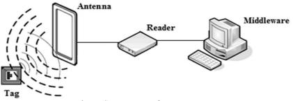
Fig. 7. Components of RFID system
